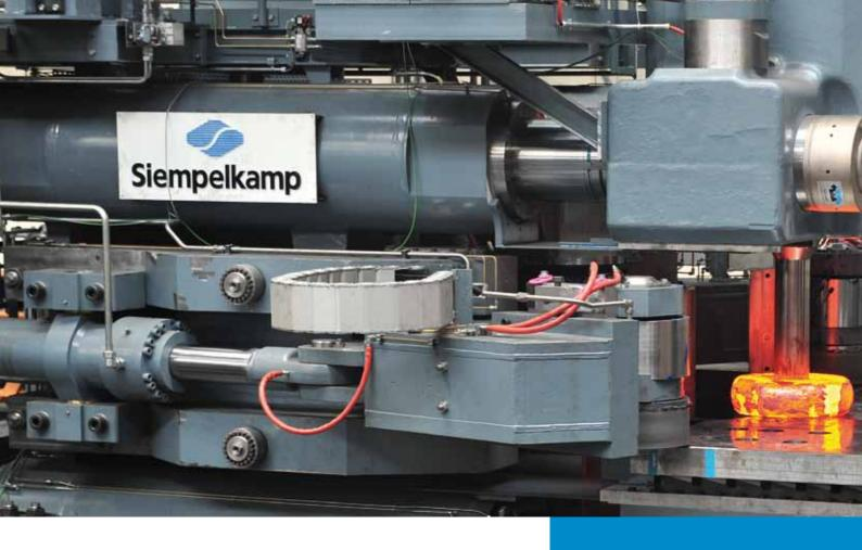
With the ring rolling mill, Siempelkamp once again demonstrates its competence as a systems supplier and provider of complete solutions which designs and builds presses for all stages of metal forming.
