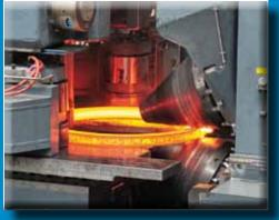
optimal ring rolling process and keeps the rolling parameters synchronized with the process. The rolling process can be completely documented and archived.
