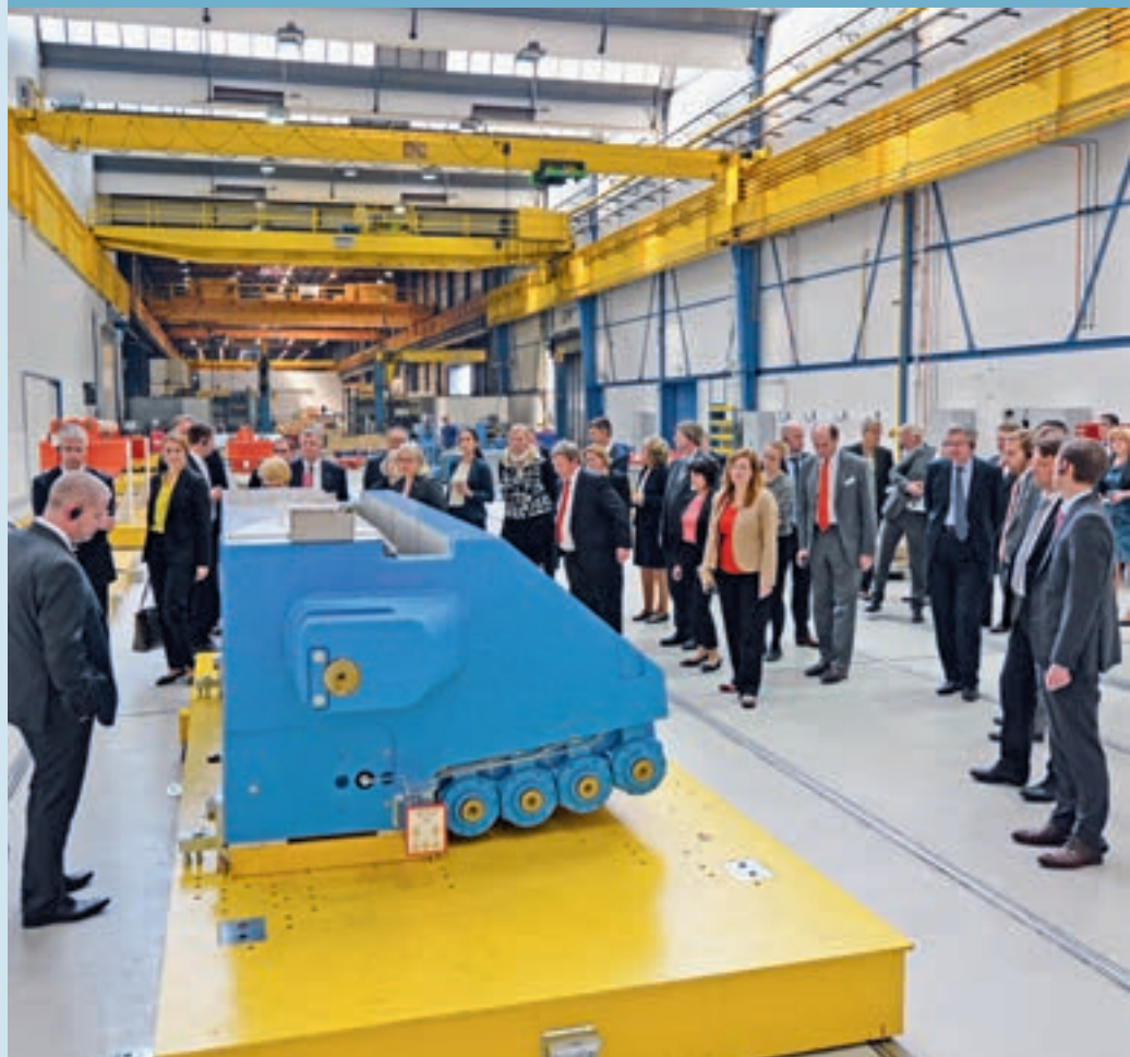
Made in Germany: infeed head – key component of the infeed section of a ContiRoll® press
