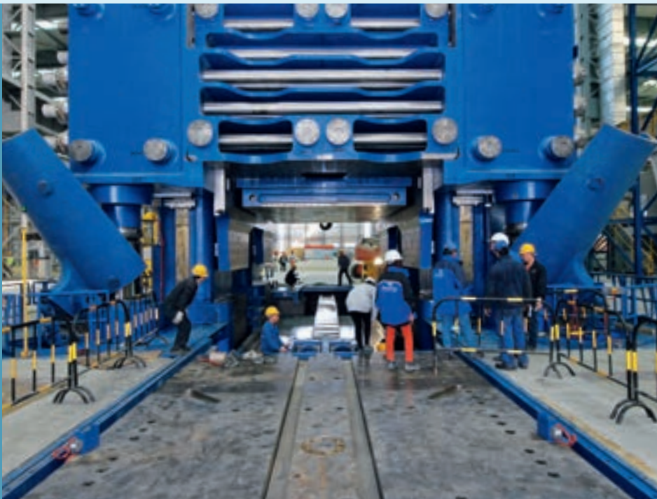
500 MN press with locking mechanism for the moving beam
