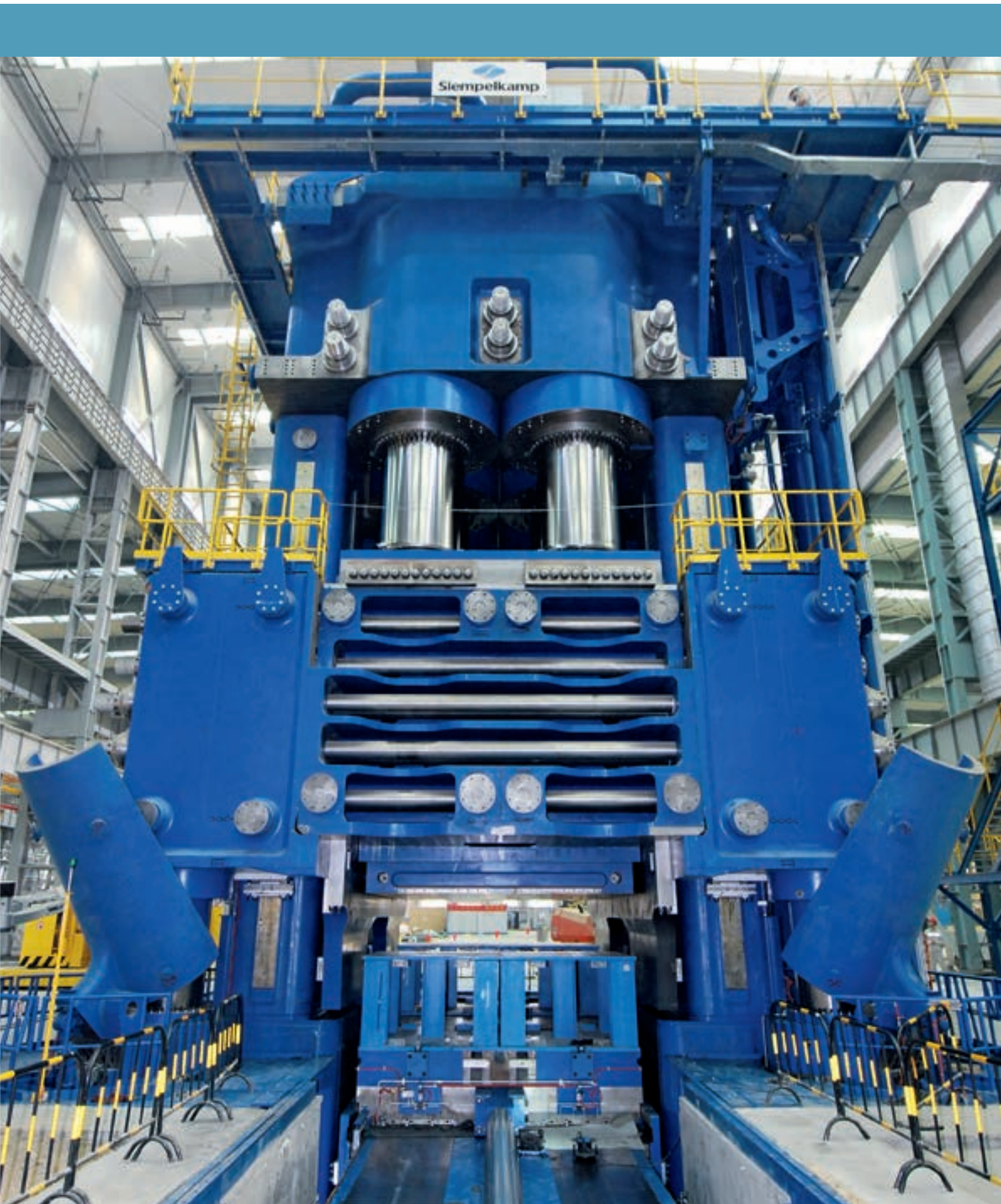
500 MN closed-die forging press of Nanshan Group
