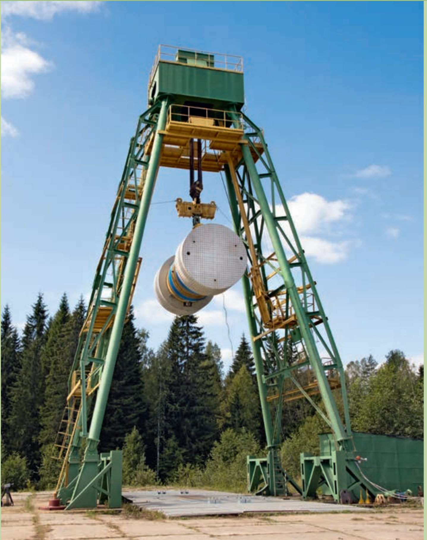
9 m drop test – for maximum safety
