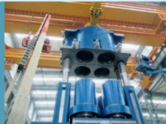
Upper bolster during closing of the 500 MN press
