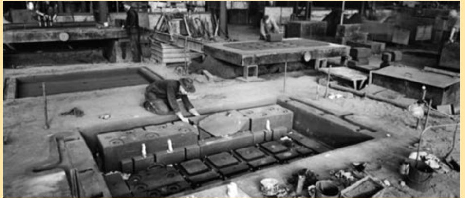
Molding a machine bed in the 1960s.
