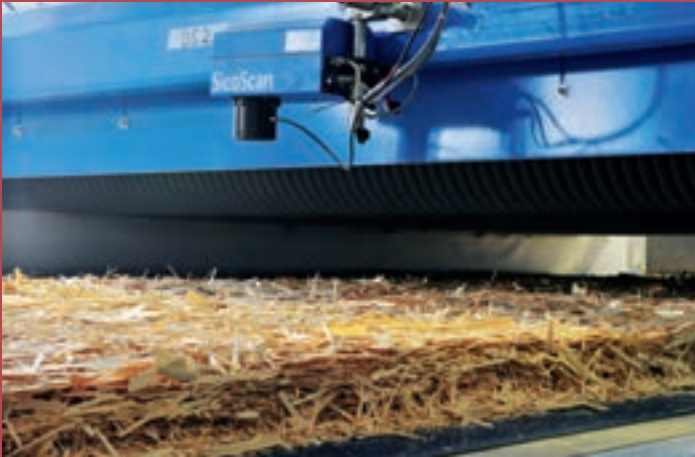
SicoScan measuring system
