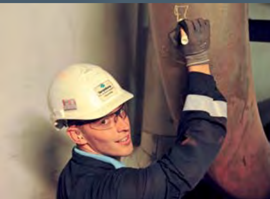
Preparatory measures for component metallography: sanding and polishing of a pre-defined measuring point
