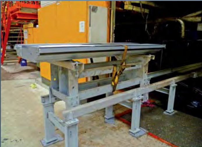
Feeding cart for pressure distribution plate segments
