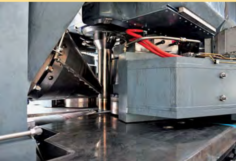
Roll table, left centering arm with 200 mm diameter mandrel
