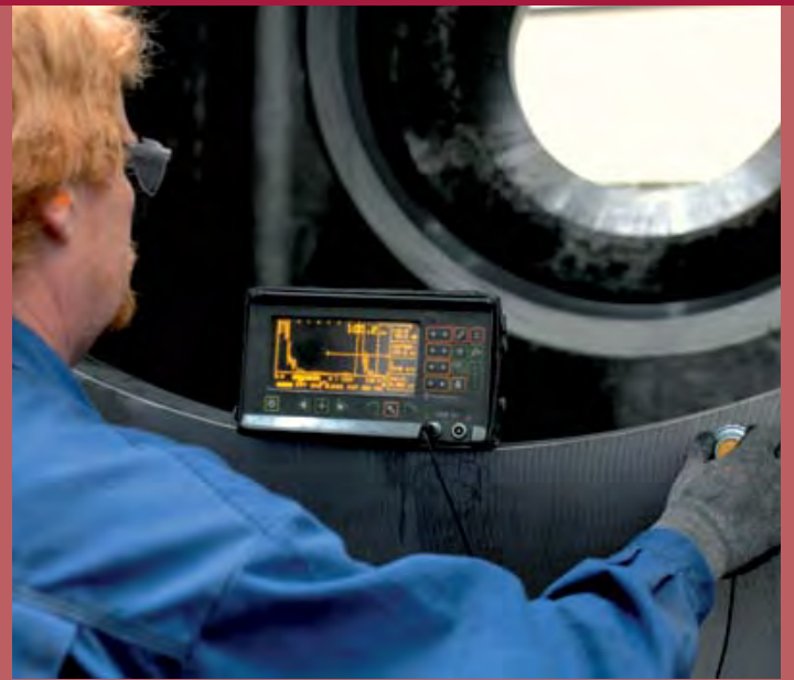
Final inspection via ultrasound
