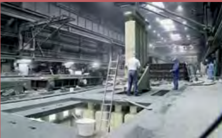
Molding shop: inserting of the cores
