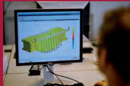
Casting process simulation
