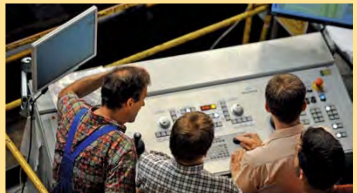
Control console for the ring-rolling mill
