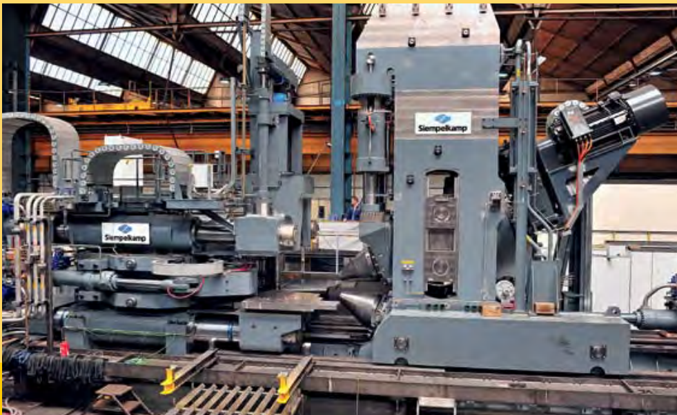
Ring-rolling mill ready for acceptance
