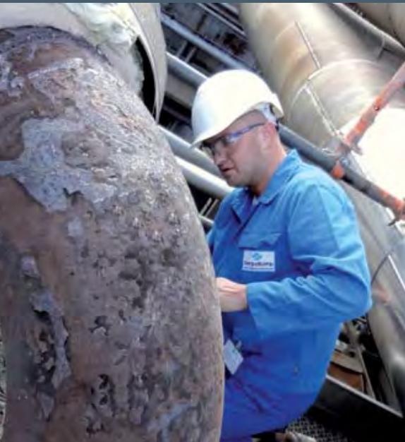
Complex inspection and assessment of remaining service life of high temperature components
