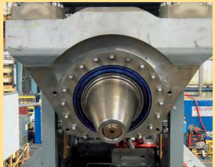
Hollow shaft with tension rod
