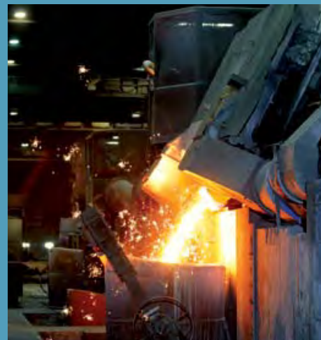
Right: Tapping: pouring of molten iron from the melting furnace
