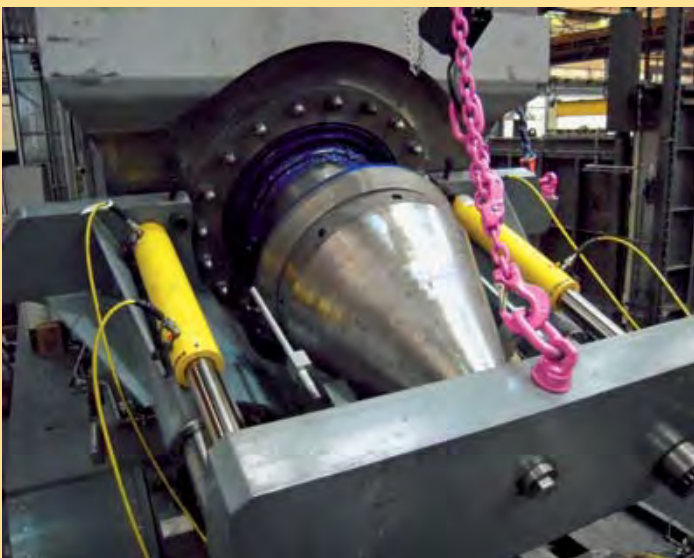
Roller cap during disassembly
