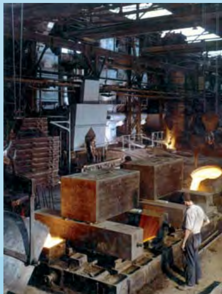
Siempelkamp Giesserei in the 1960s: cupola furnaces were used (which can be seen behind the casting setup)
