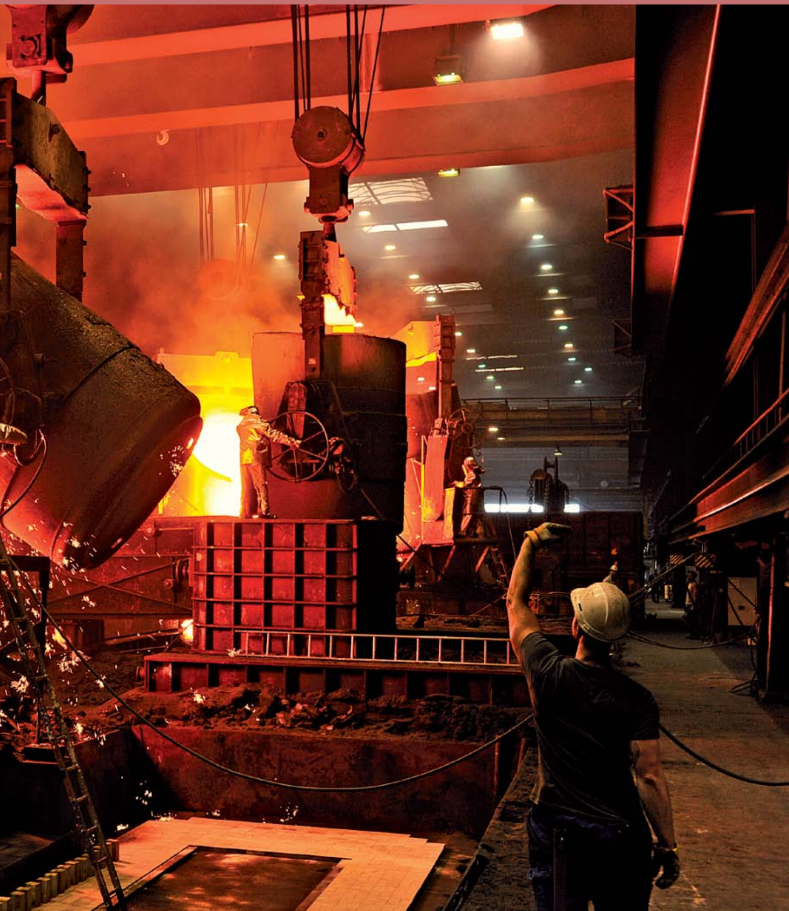
World record casting: 320 t lower press beam for the 125 MN Nanshan press
