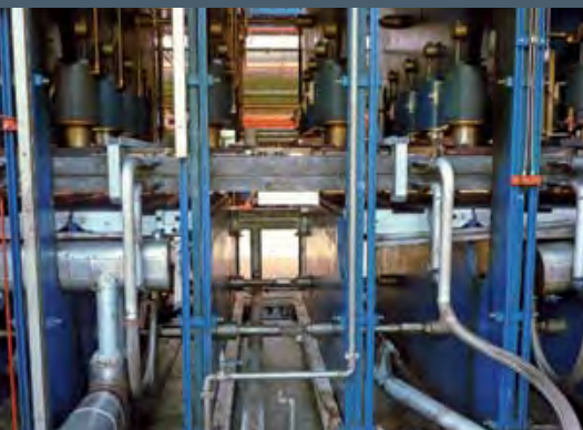
Raised hot plate with inserted pressure distribution plates
