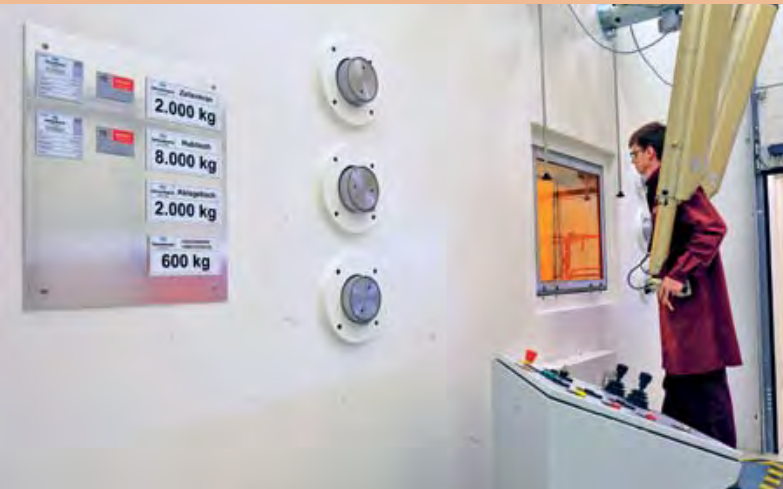
Easy handling: remote handling of the hot cell at the handling center of the NES
