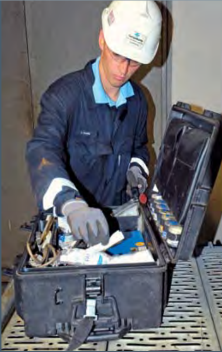
Inspection box for ambulant component metallography
