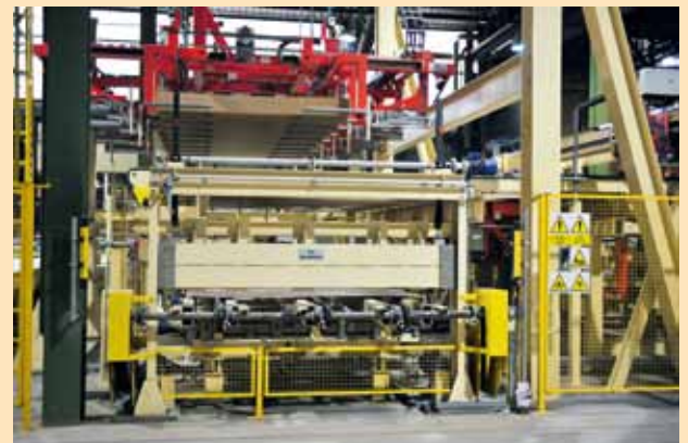
Top: Vapor exhaust Bottom: Stacking with cover board feed
