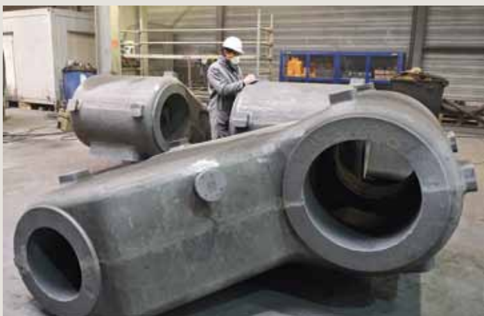
Quality inspection of the wing arm cast component for use in cement mills
