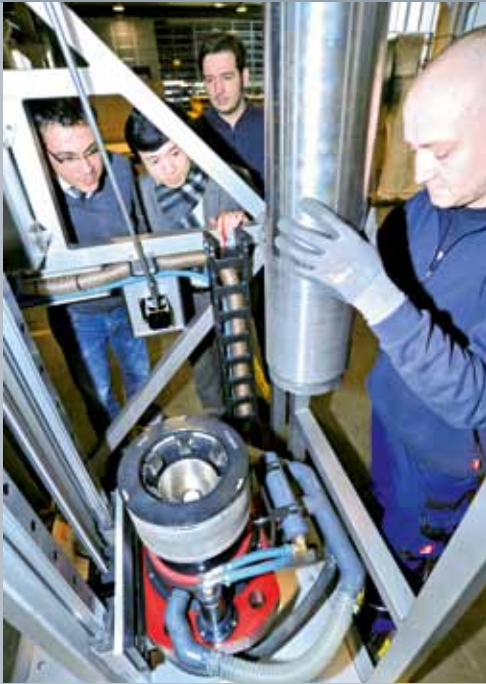
Functionality test at the STS in Lünen, Germany: a bolt is placed into the cleaning head
