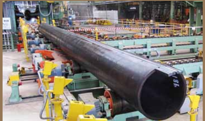
Slot pipe after O-ing
