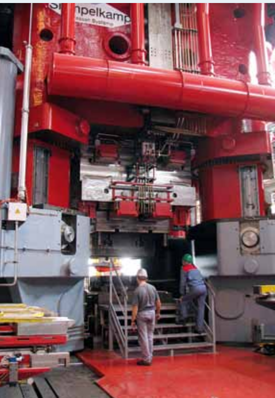
40,000 t press for the production of structural components for the aerospace industry
