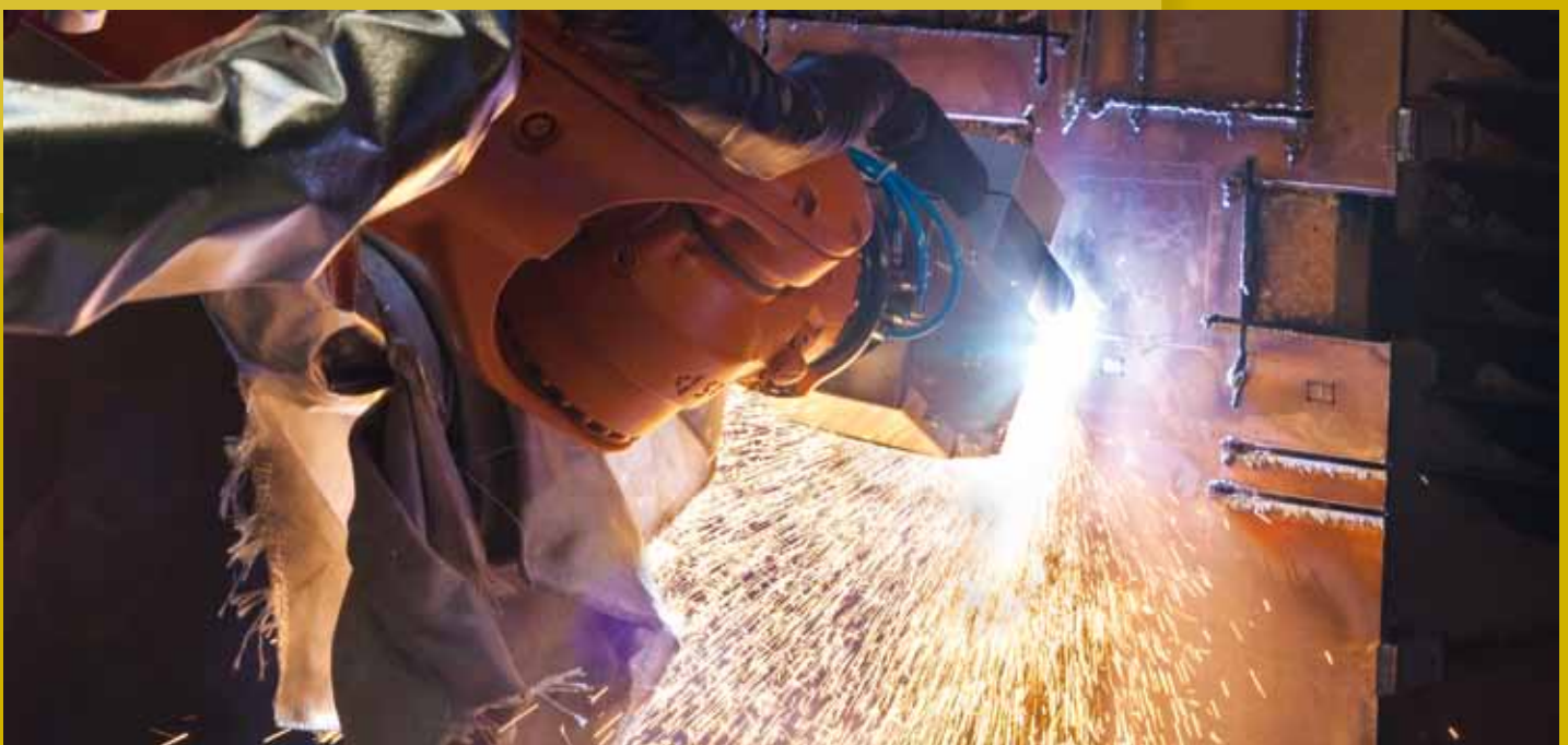
Testing of the hot wire process: performing of various flame cuttings
