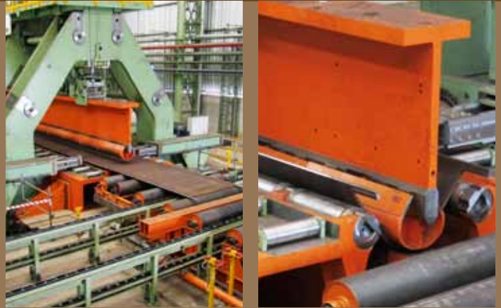
Left: Crimped plate in front of the U-forming press Right: U-forming
