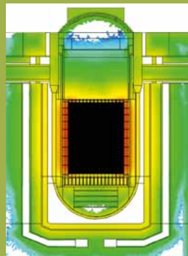
Presentation of the reactor neutron intensity distribution in a cut-out of the 3-D model of the upper reactor pressure vessel and the loop pipe: red = higher neutron intensity and thus higher activity.
