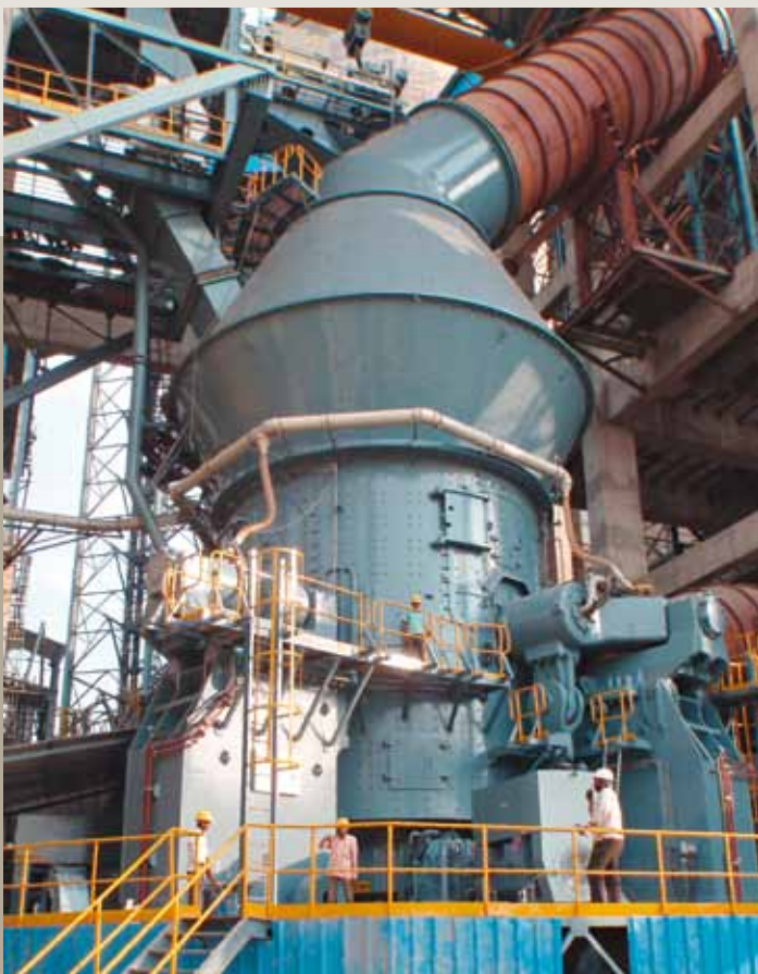
PFEIFFER vertical roller mill MVR 5600 C-4 for cement (photo: GEBR. PFEIFFER SE)
