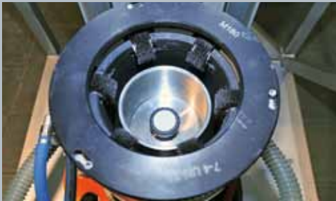
Interior view of the cleaning head, equipped with six stainless steel wheel brushes for cleaning the thread sections of the bolt
