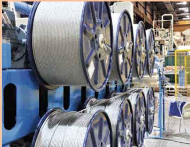
Left: Spools with direct tensioning drives, Right: Tension measurement device
