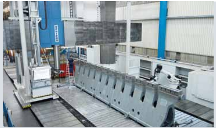
Upper die during mechanical machining at Siempelkamp
