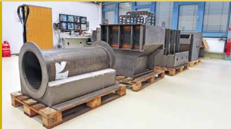
Realistic test specimens at the NIS Technical Center to test the hot wire cutting process
