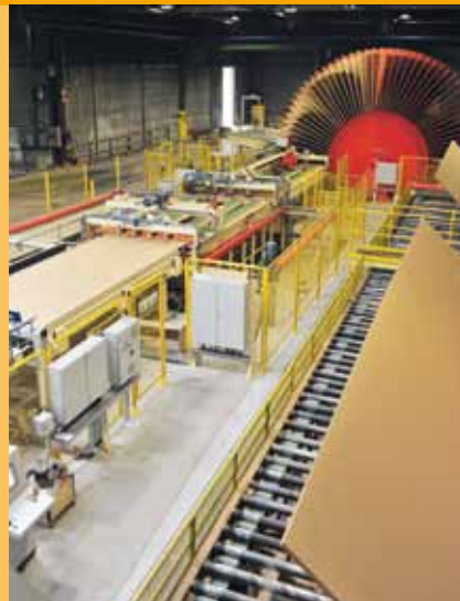
Removal of thin boards
