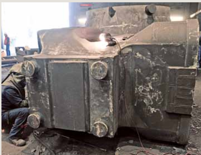
SACMI cross beam receives the final finish at the fettling shop
