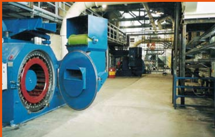
Links: Messerring-Zerspaner Rechts: Rotor HMT
