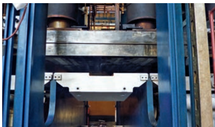
Subsequent installation of pressure distribution plates in an existing press
