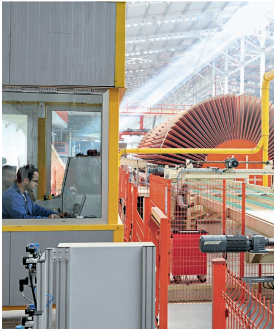
..... Finishing line with cooling turner .....
