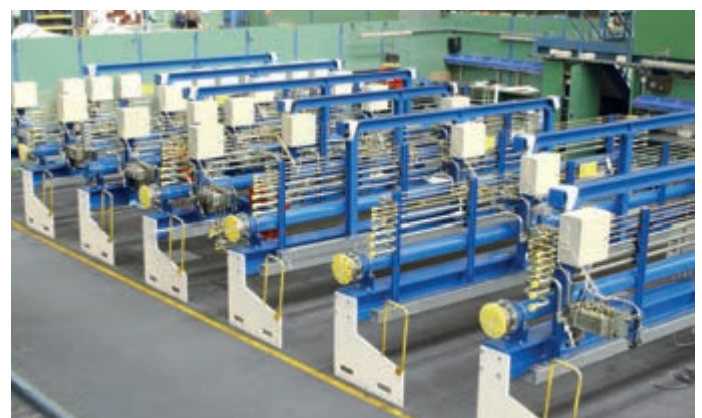
Hydraulic function carrier with 6 m length
