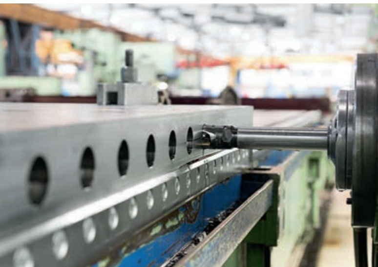
..... Deep-hole drilling of channels of a hot platen .....
