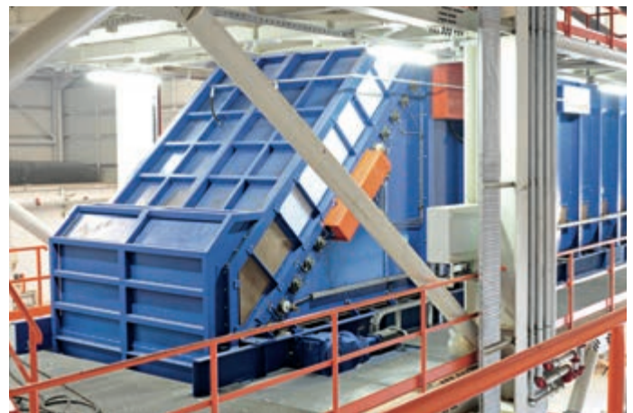
..... Edge trimming of the fiber mat Frontal discharge of the mat former bunker .....
