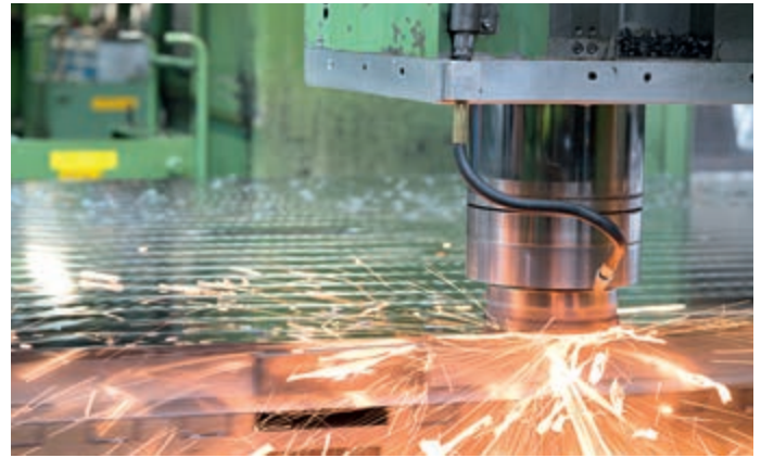
Precision-milling a hot platen Assembly work on hydraulic components
